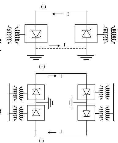
Each terminal has two sets of converter of identical ratings in series on the DC side. The junction between the two sets of Conductors is grounded at one or both ends.
