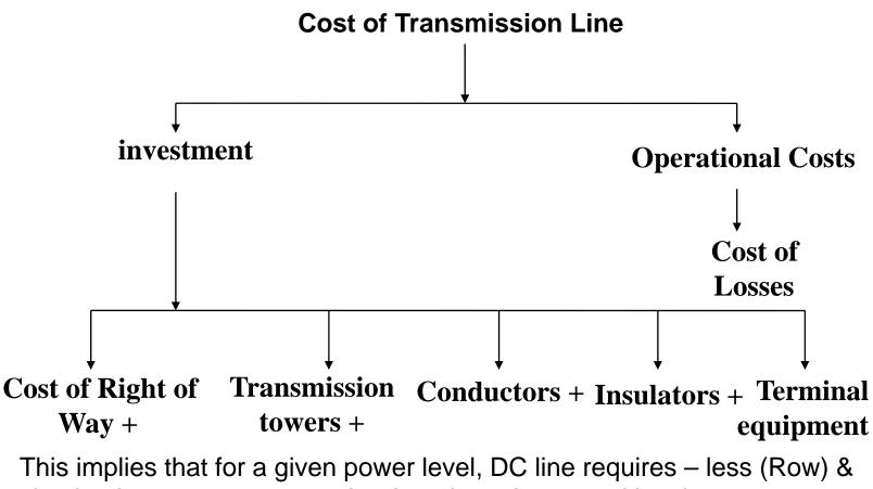
simple-cheaper towers - and reduced conductor and insulator costs.
